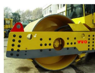
Heavy duty vibratory rollers are suitable for compaction of non-cohesive materials such as gravel, crushed stone, sand-macadam mixture, sandy soil and rock filling etc. on bse course sub-base and embankment fill construction etc., which are ideal equipment for high-class highway, railway, airport, harbors, dams and large-scale industrial ground etc.
